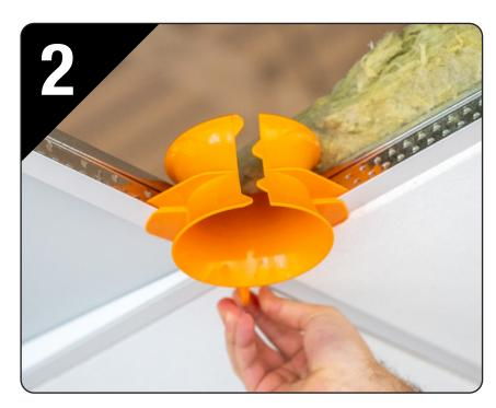
2. Slide the Cable Funnel into the corner of the ceiling grid, positioning the upper tabs above the grid and lower tabs below the grid.
